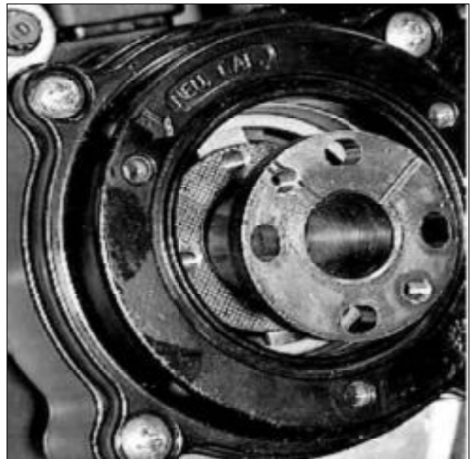
Fig. 7-11 . Vertical witness mark alignment.
