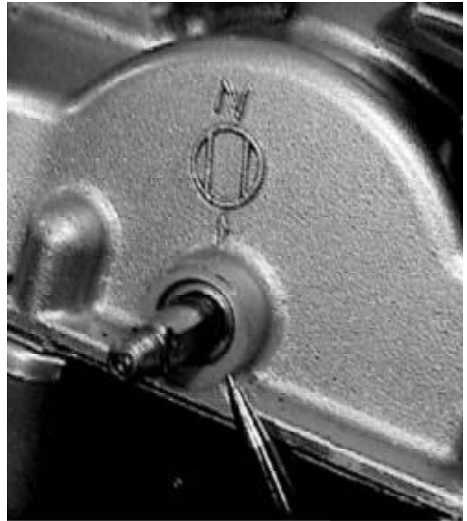
Fig. 7-4. NBSU alignment marks.
