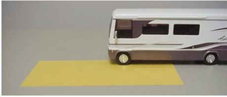
Weighing Left Front 'Corner'
