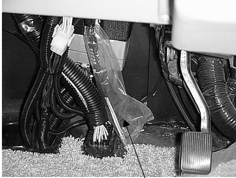
CB Wires (in plastic sheath)
