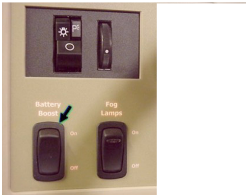
Battery Boost Switch
