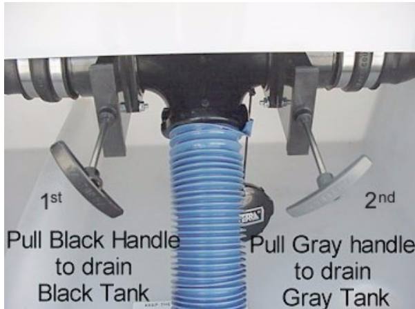
Holding Tank Valves (Typical)
