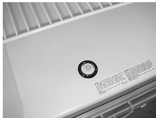
Place bubble level in bottom of refrigerator
