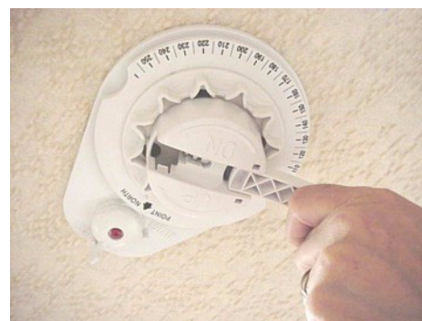
Digital Satellite Dish Control located on ceiling
