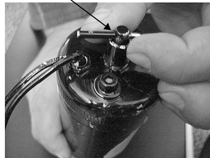
Leveling Jack Solenoid Valve
