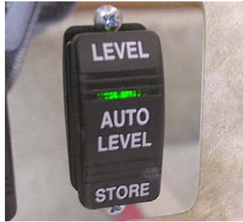
Auto Level Switch (Located inside entrance door)
