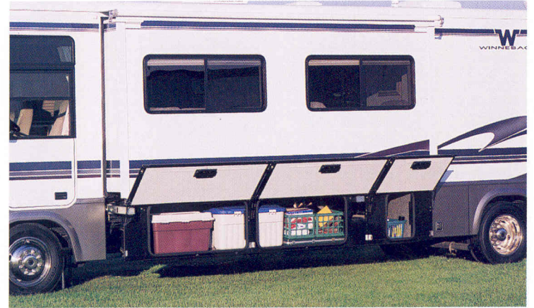
37G The StoreMore™ Hydraulic Slideout System gives you extra living space without sacrificing storage space. The generously sized compartments move with the room itself, offering easy access to stored gear.
